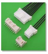
XAF connector is an insulation displacement socket connector which is compatible with the existing XA connector crimp housing (plug housing). The dipping type, SMT type, and high box type headers or the receptacle housings used for wire-to-wire connection can be prepared as the mated counterpart of XAF connector, and the wide range of connection style can be provided depending on the application application.
