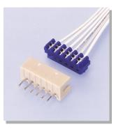
2.0 mm pitch IDC type CR connector enables to terminate with UL 1007 wire used for internal wiring of equipment specified in the Japan Electrical Appliance and Material Safety Law. This connector has a low-profile design with a mounting height of 6.9 mm and a thickness of 4.8 mm (in case of top entry type).
