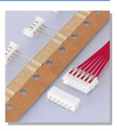
This thin type 2.5 mm pitch connector is an IDC style for PC boards. It is developed by integrating the technologies of crimp style connectors such as EH and PH, and IDC style connectors such as NR, DR, and DB. The In-line method that the wire extraction direction is perpendicular to the board provided high density wiring provides high-density wiring.
