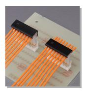
The VR series is a 3.96 mm pitch wire-to-board connector for 7 A rated power supply circuits. Furthermore, it can accommodate AWG #18 wire, which is rare for an IDC connector.
